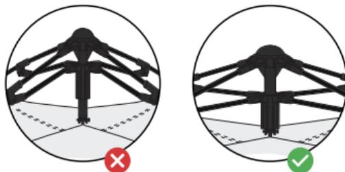
2. Stand at the back of the tent, lift the upper support pole of the tent up. Then press the support pole down here.
